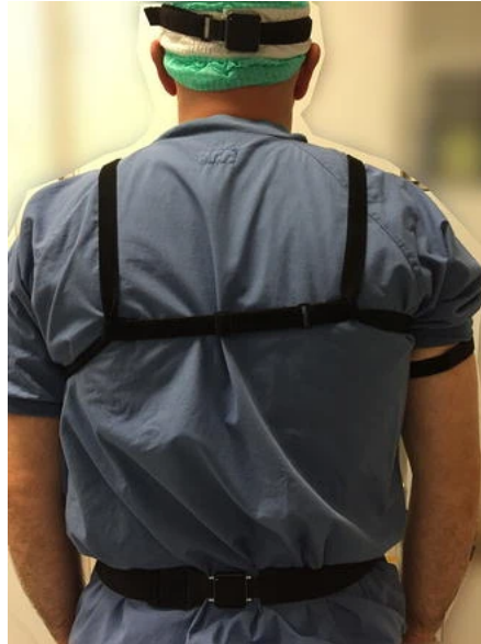
Figure A-2: Placement of IMUs on surgeon on the back of the head, the sternum, upper arms and pelvis. (85)
