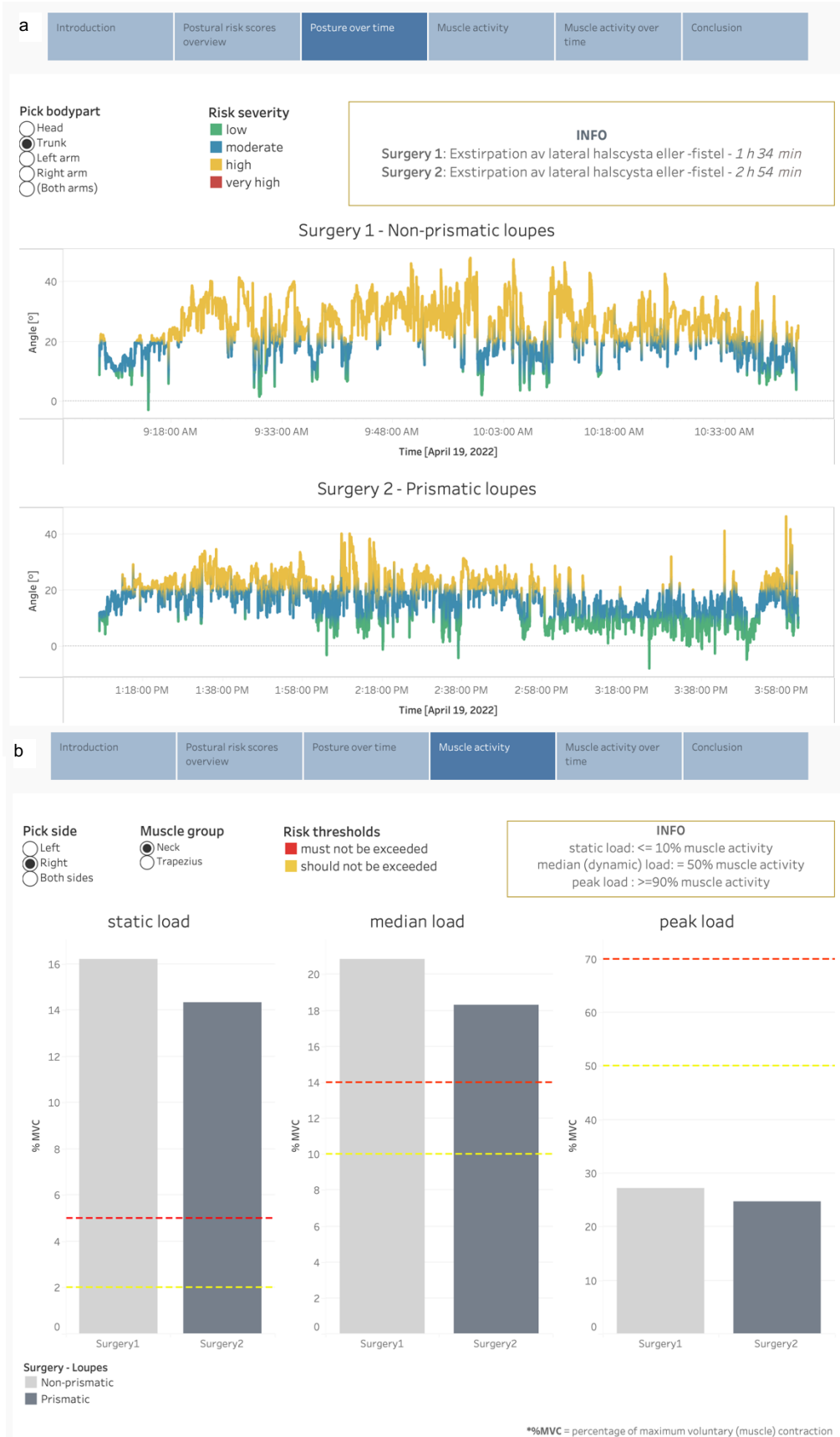
Figure 3-2 Tableau sheets of ergonomic report: a) postural angles over time; b) muscle activities in different load levels
